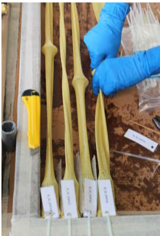
Figure 7: Forming process by manual fabric manipulation introduces qualities of craft into the industrial setup of composite manufacturing
