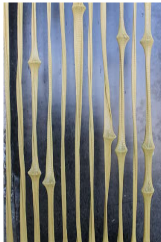
Figure 8: Variants of knit element (type:3000D), created by the simple placing of tension rings
