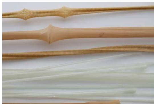
Figure 5: Five types of elements were manufactured: 2 types of para-aramid knitting and 3 types of fibreglass sleeves of different diameters
