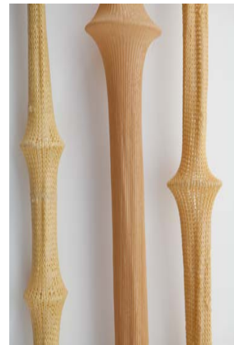
Figure 6: Stoppers created through local deformation of the sleeve by the insertion of rings under tension (Photo: Amit Ofek)
