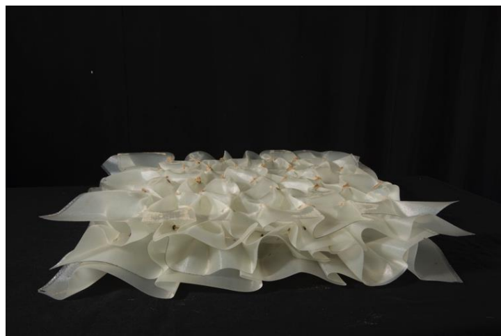
Figure 1. Layered FM-FRP material system (L-FMFRP) resulting in architected material shaped as a thick panel.
