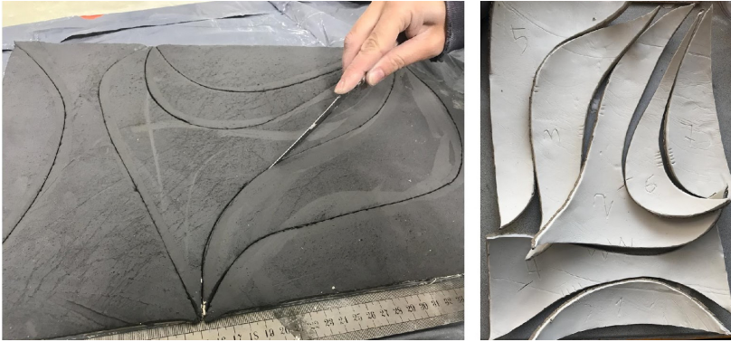
Figure 9. From flat sheets to shaped ceramic, illustrating geometrical incompatibilities: the matching curves in the flat sheet transform to non-matching edges once frustration is in play.
