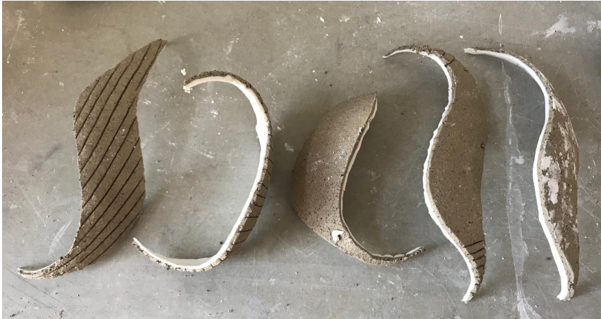
Figure 11. Oscillating curvature of two-dimensional contour curve creates significant displacement in resulting surface. Grooves on the terrazzo layer enable additional displacement and curvature.
