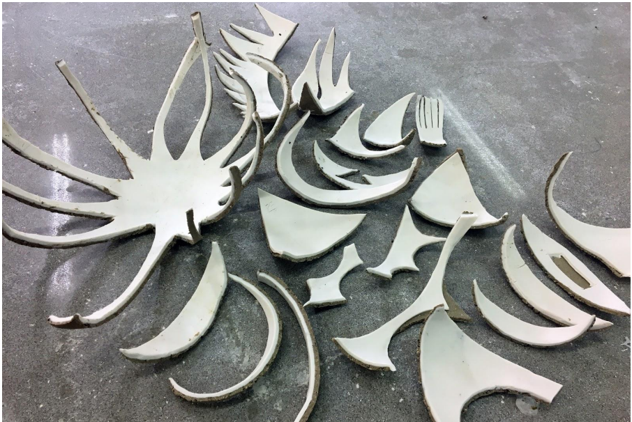
Figure 7. Series of ceramic material exploration, seeking to accentuate displacement and curvature of the ceramic surface, observed as maximal Z value and minimum radius of curvature
