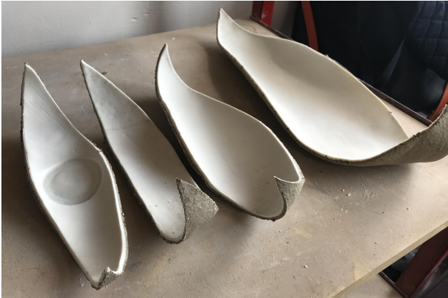
Figure 10. Prioritising long and narrow shapes where lateral frustration is reduced, and significant curvature can take place in the long direction.
