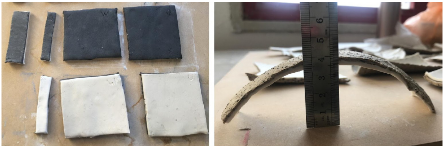
Figure 8. Flat rectangles of ceramic-body entering the kiln for drying and firing (b) resulting three-dimensional shape.
